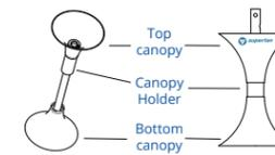
Insert the bottom canopy (one without the logo) through the downrod. Place the canopy holder on top of the bottom canopy such that it rests on the inner step of the canopy. Now insert the top canopy (one with the logo) through the downrod and pull it down through the canopy holder until it is obstructed by the bottom canopy. The top of the downrod must be visible as shown in the figure.
