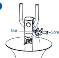
Fasten the other piece of the metal clamp onto the looped piece using the screw and nut to secure the safety rope. Fold the free end of the safety rope back into the downrod from the top and raise the canopy to the ceiling.
