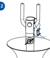
Loop through the ceiling hook and pass the free end through the other pair of holes in the same piece of the metal clamp. Leave a slack on the loop so the fan is not supported by the safety rope alone.
