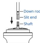
Fix the slit end of the downrod tightly onto the shaft using the bolt, washers, spring washers, and nuts.
