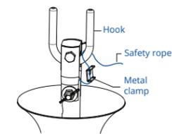
After the fan is secured by the shackle kit, pass the safety rope through one pair of holes in one piece of the metal clamp as shown in the figure.
