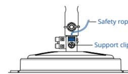
In the safety rope assembly, unscrew the metal clamp to part it into two pieces, and unwind the safety rope. Pass the un-beaded end of the safety rope through the support clip from bottom to top. Pull out through the support clip until the beaded end fastens to the support clip.
