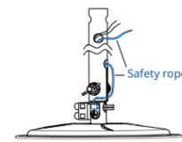
Insert the free end of the safety rope through the hole in the downrod that is free from wires. Push the safety rope through the downrod and pull it out from the hole on the side of the downrod at the top.
