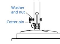
Insert the cotter pin through the bolt hole and bend its ends to fasten it.
