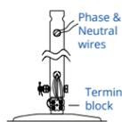
Insert the phase wire (usually red) and the neutral wire (usually black) through the hole on the side of the downrod at the top. Pull them out of the slit and connect them to the terminal block.
